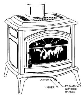
PUSH IN ALL THE WAY (TO RESET CONTROL PLATES), THEN PULL OUT IN INCREMENTS TO DESIRED HEAT OUTPUT SETTING.
